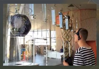
The higher the concentration level the faster the fan spins and the "world" is lifted
